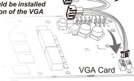
Hold the VGA card and have the gold finger side face toward you with the VGA card facing downward. Insert the first spring loaded screw through the Omni-Mount Backplate and through the VGA card
