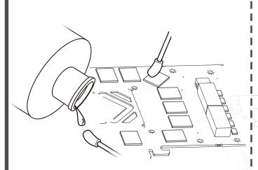
Before installing heat dissipation plate, clean the chip surface with ethanol to remove oil film or stain which may block heat transmission, so as to enhance adhesion of heat dissipation plate.
